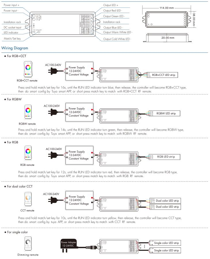
Press and hold match/set key for 8s, until the RUN LED indicator turn white, then release, the controller will become DIM type, then do smart config by Tuya smart APP, or short press match key to match with dimming RF remote.
