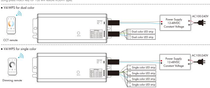
Note: The output power of a constant voltage power supply should be at least 1.2 times that of the output load (light strip), otherwise the full power output of the load can easily cause automatic flickering or shaking of the light.
