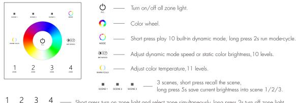
1 2 3 4 20NE Short press turn on zone light and select zone simultaneously, long press 2s turn off zone light. Short press multiple zone key fastly, will select multiple zone synchronously. 4 zone control seperately or synchronously, each zone could control multiple receivers.
