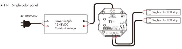
DIP switch select four PWM frequency: 1KHz, 2KHz, 8KHz or 16KHz. Higher PWM frequency, will cause lower output current, higher power noise, but more suitable for camera(No flickers for video).
