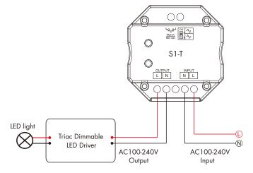
Note: When calculating the maximum number of load lamps or drivers, the input power or input current parameters of a single lamp or driver must be used, the output power parameters can not be used.
