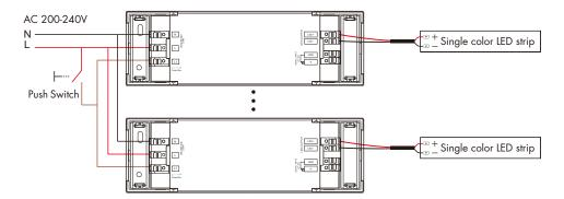
The provided AC Push-Dim interface allows for a simple dimming method using commercially available non-latching (momentary) wall switchs.
