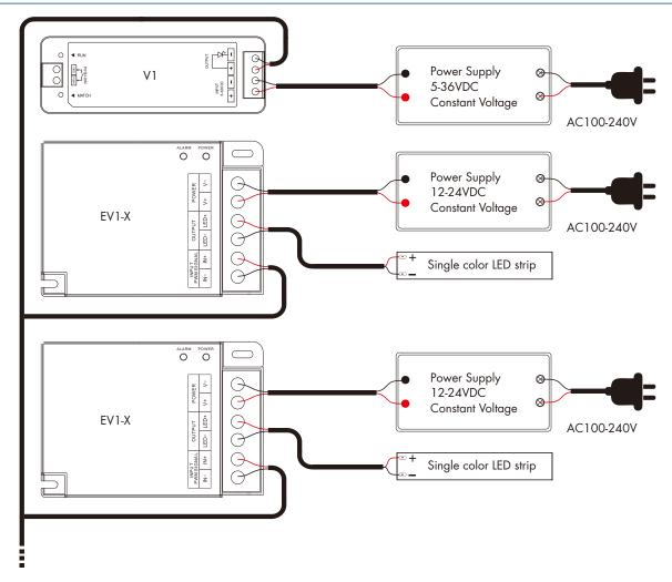
Note: If the power repeater is over heat, over load or short circuit, the ALARM LED indicator will blink.
