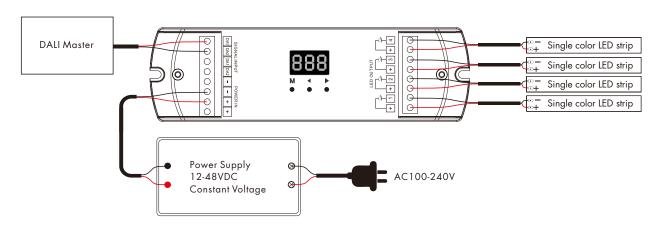
Note: When display OLA, overload alarm. When display OHA, overheat alarm.
