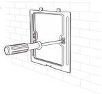
5. Slant the switch plate cover and put it in place, then secure the plate cover to the switch from the bottom with a KM2 screw.
