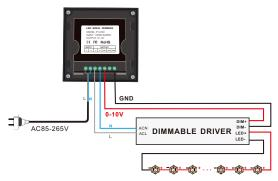
\*\* The dimmer will automatically cut off the output voltage when the brightness signal is 0%, and stop powering the dimming power. With this function, it can solve the problem that some dimmer power couldn't be turned off through dimmer signal.
