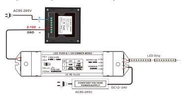
For the dimmer driver or dimming power which can be completely turned off only via dimming signal, can connect only the dimming signal of dimmer, without using other voltage output.
