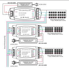
2) with power amplifier the controller and the amplifier can share the same power supply:
